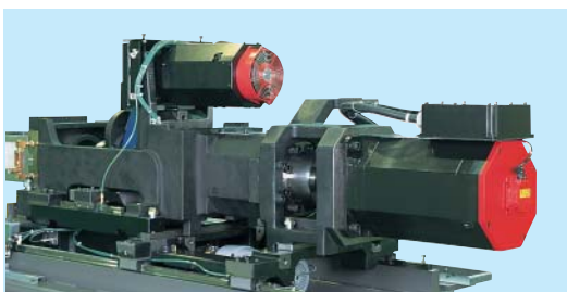
Motor directly coupled injection mechanical unit (option)
