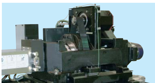
High rigid and low friction injection mechanical unit
